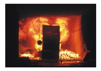
The Applus+ TST technological centre in Asturias (Spain) is equipped with a specialist test tunnel designed to reproduce the conditions of a full-scale fire in a confined space such as a tunnel, shaft, mine, ship or other underground structure.
