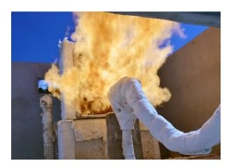
The storage and transport of hydrocarbons and other chemical products in plants, tanks, pipes and vessels call for extremely strict fire-protection measures. As these inflammable products are stored under pressure, any leak could result in a virulent fire with a high rate of flame spread. For this reason, **passive fire-protection products aimed at the oil and gas or marine industry** must pass specific tests that simulate the extreme conditions they would face in the event of a fire.
