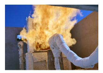
The storage and transport of hydrocarbons and other chemical products in plants, tanks, pipes and vessels call for extremely strict fire-protection measures. As these inflammable products are stored under pressure, any leak could result in a virulent fire with a high rate of flame spread. For this reason, **passive fire-protection products aimed at the oil and gas or marine industry** must pass specific tests that simulate the extreme conditions they would face in the event of a fire.
